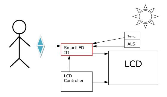
Figure-1: Overview of SmartLED-II usage (ALS = ambient light sensor)
