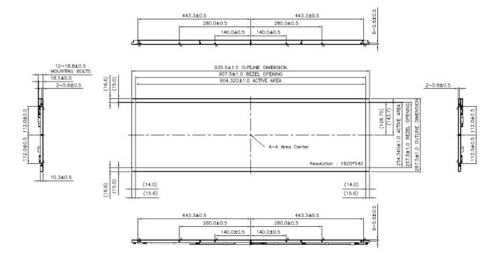
A M3 MOUNTING HOLE (14X) DP=4.0mm MAX SCREW
