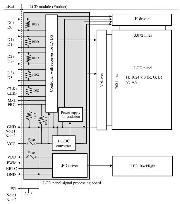
Note1: Relation between GND (Signal ground and LED driver ground) and FG (Frame ground) in the LCD module is as follows.
