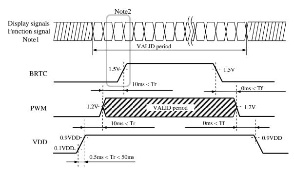
Note1: These are the display and function signals for LCD panel signal processing board.
