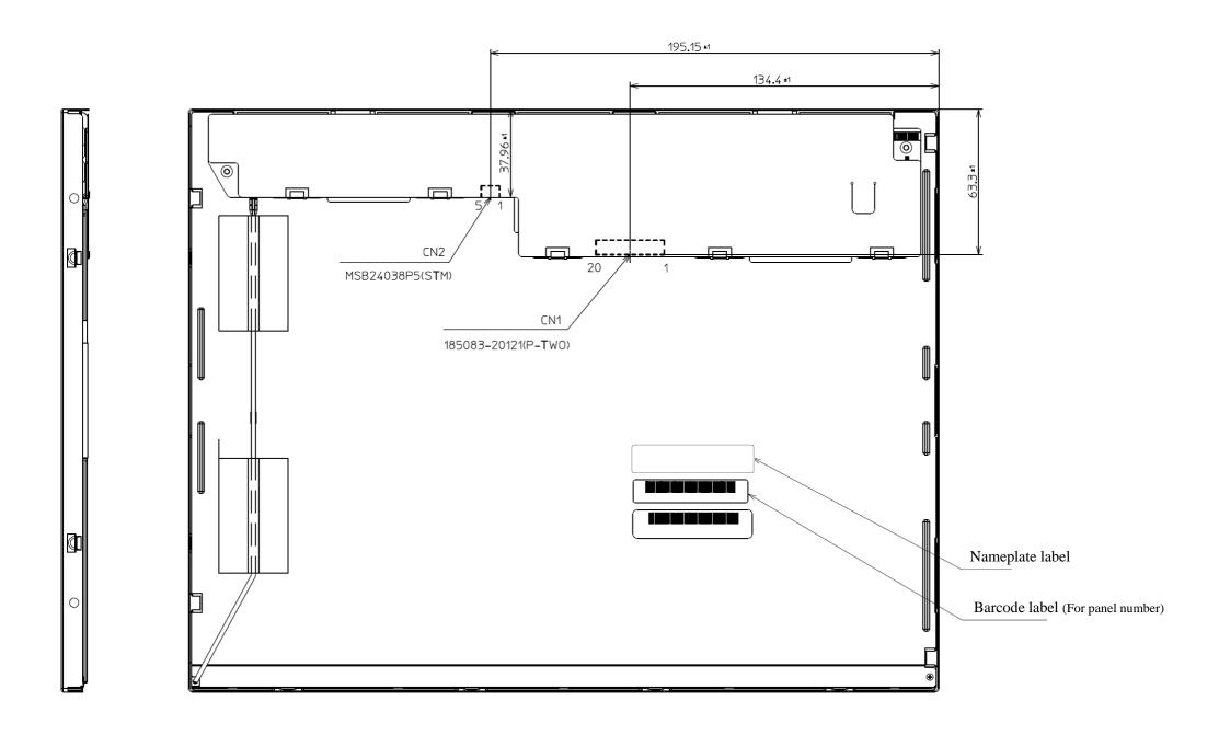
Note1: The torque for product mounting screws must never exceed  $0.392N \cdot m$ . And the length of product mounting screws must be  $\leq 4.5 \text{ mm}$ .
