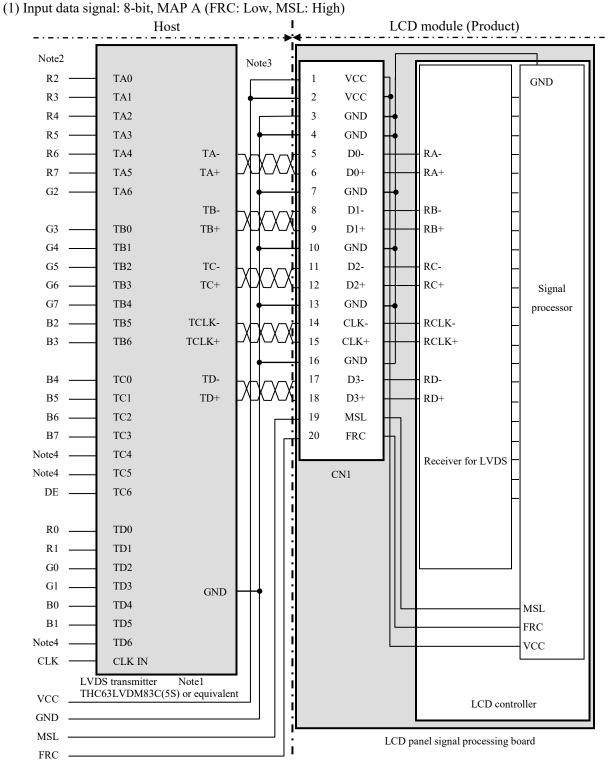
4.5.4 Connection between receiver and transmitter for LVDS
