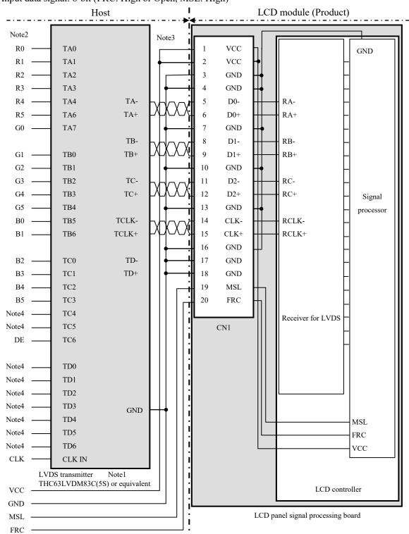
(3) Input data signal: 6-bit (FRC: High or Open, MSL: High)
