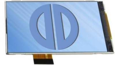
Same 3,2" TFT display without protective glass: the very small bezel and the fragile mechanics do not allow for tape assembly or wet bonding
