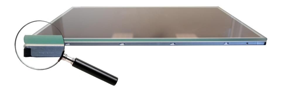
Free-air-exclusion TFT Display with protective glass optically bonded with VacuBond®
