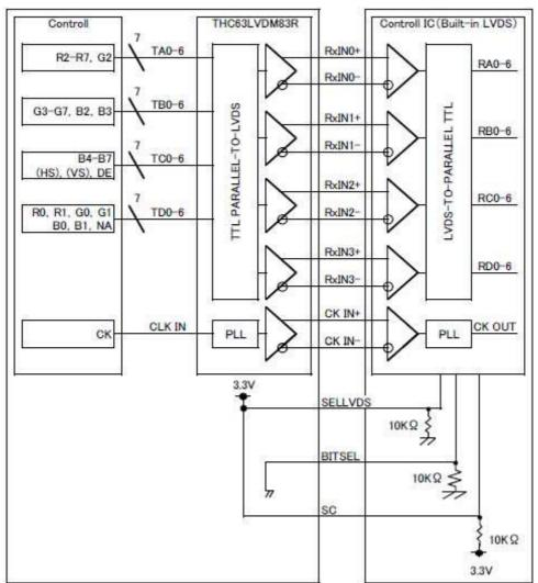
$\mbox{\ensuremath{\mbox{\$}}}\mbox{SELLVDS}$  signal line has 10 k  $\Omega$  -pulldown resister.
